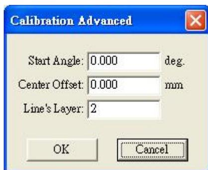
**Start Angle** Set the angle of the first scale line, namely the initial rotary point
